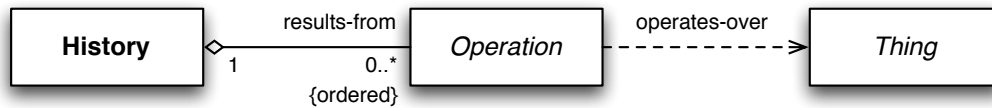
Figure 4: Class diagram of the HISTORY OF OPERATIONS pattern. A History results from a set of Operations done over Things.
